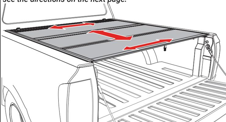
**12** The rear edge of the cover (A) and tailgate seal should rest on top of the tailgate. **You are ready to drive with your cover in the closed position.**
