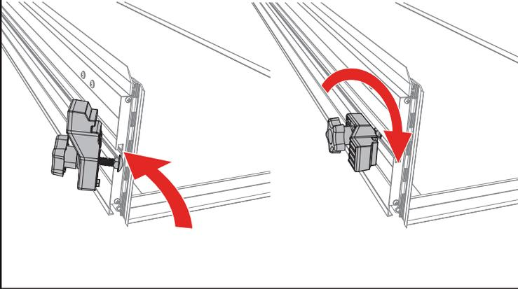
**8** Position the buckle ends (I) with the open side facing the bed cover panel. Use a screwdriver to install the two buckles into the pre-drilled holes on the front header panel with the provided screws (J). **DO NOT use a screw gun, securely tighten by hand only.**
