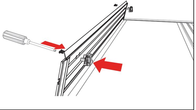
**9** Set the cover (A) in the folded position on the side rails (B & C) towards the cab of the truck. Confirm the cover is evenly spaced between the rails.
